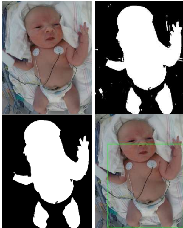
Figure 4.5: First row: original and binary images; second row: filtered binary image and ROI.
