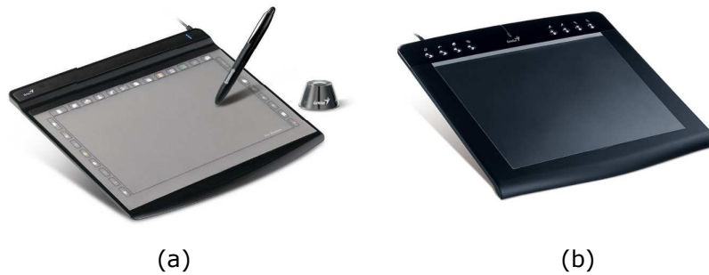
Figure 3.11: The two graphic tablets used as absolute positioning systems for the experiment with TAMO1 (a) and TAMO3 (b).
