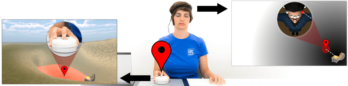
Figure A.3: The complementary feedbacks of our haptic system: vibrotactile HMD egocentric representation(right) and TAMO3 allocentric one (left).
