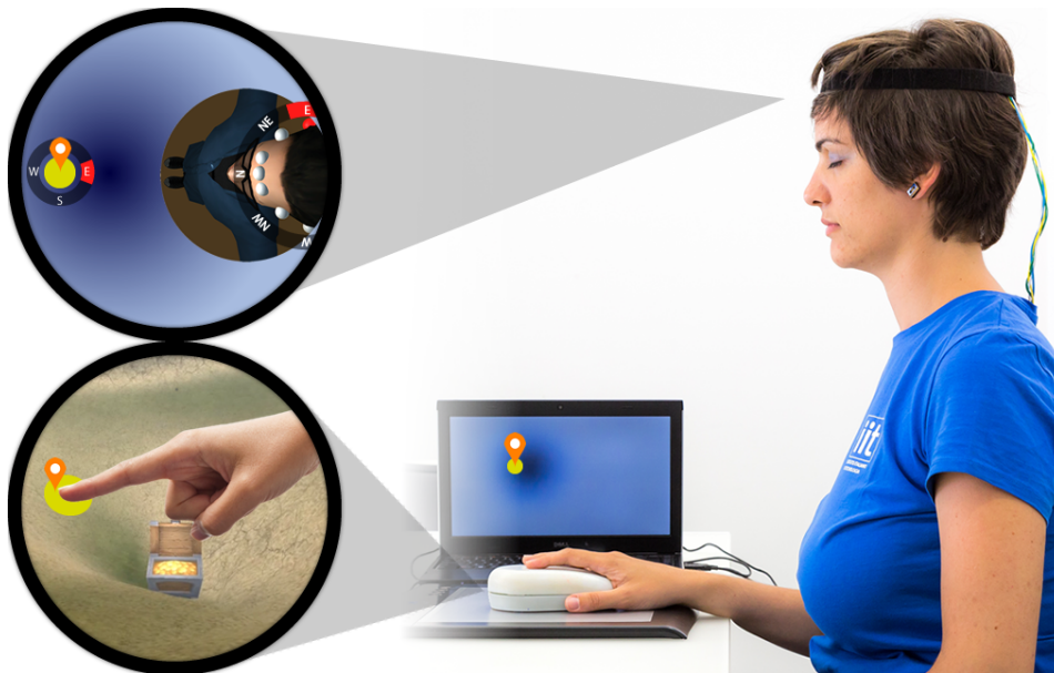
Figure A.2: Haptic system composed by the TActile MOuse 3 (TAMO3), and a vibrotactile HMD. While the TAMO3 supports the exploration of tactile maps from a top-view, the vibrotactile HMD provides an ego-referenced directional cue updated as a function of the TAMO3 movement.
